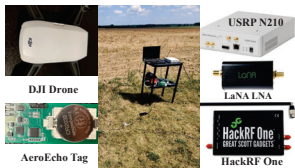
Fig. 8. Implementation of the excitation source, tags, and gateway in the farm.
